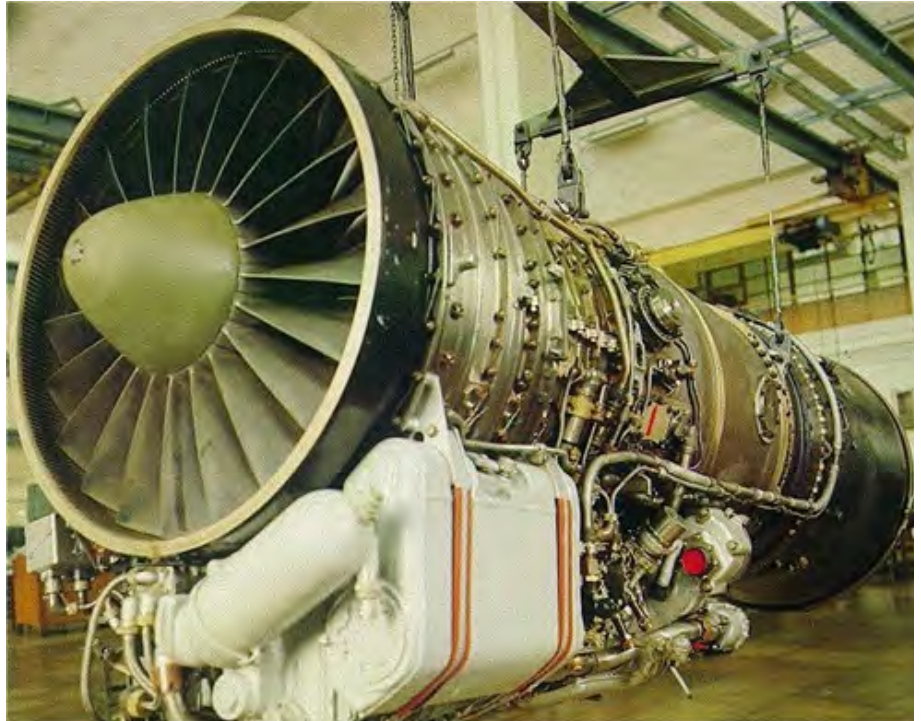
▲ MIDHANI developed and supplied Nickel Based Super alloy for MiG Engine Programme
